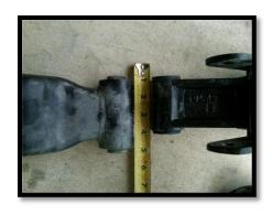
Determine if your truck has a stock shackle of 4" or 41/2". If so, ask for the ½" steel separator that is installed in the frame side, **Two** steel separators are needed for 4" and four steel separators for 4 ½" width.
