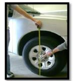
3. Using a tape measure, record the distance from the ground to the place on the fender that is directly above each tire. MAKE SURE THAT THE TAPE INTERSECTS THE CENTER OF EACH TIRE. AT THE AXLE.
